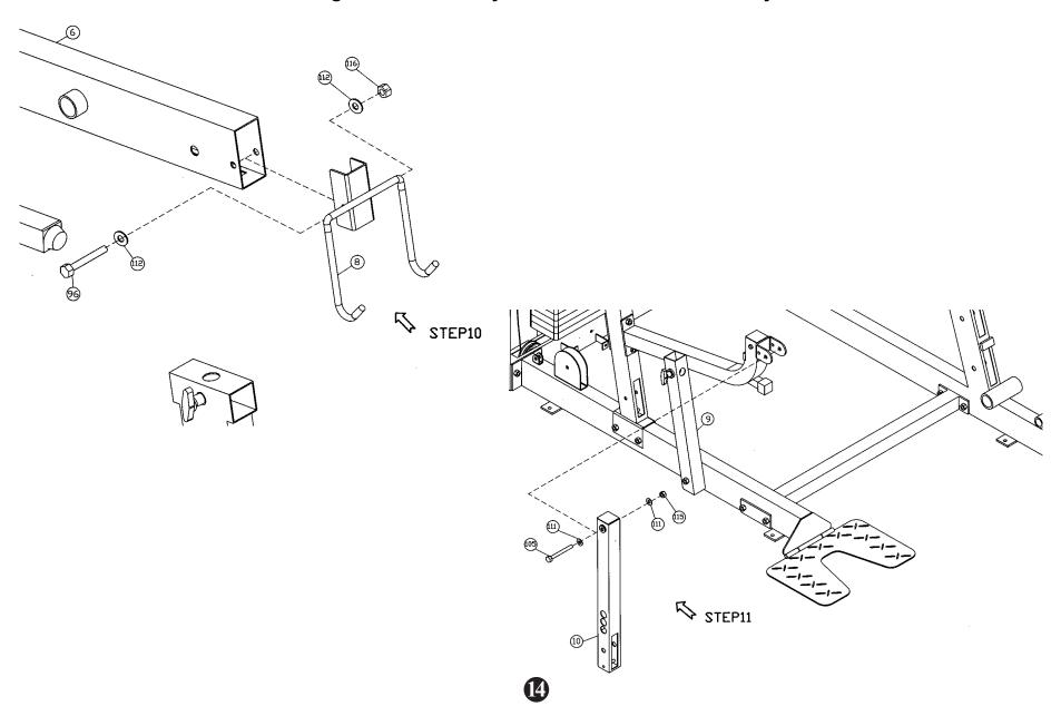
NOTE: Hand tighten bolts and nylon nuts until machine is fully assembled.
